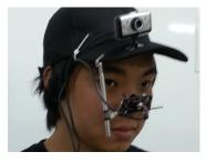
**Figure 2:** Low cost wearable head mounted eye tracker.
